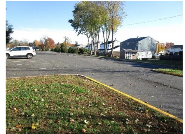
A row of parking spaces can be replaced with pervious pavement to capture and infiltrate stormwater. Bioretention systems can be installed to capture, treat, and infiltrate runoff from the surrounding paved surfaces. A preliminary soil assessment suggests that the soils have suitable drainage characteristics for green infrastructure.
