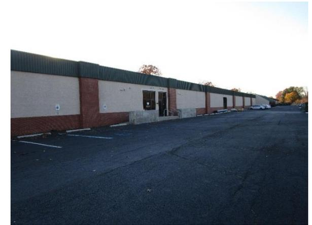
Parking spaces can be replaced with pervious pavement to capture and infiltrate stormwater. A preliminary soil assessment suggests that the soils have suitable drainage characteristics for green infrastructure.
