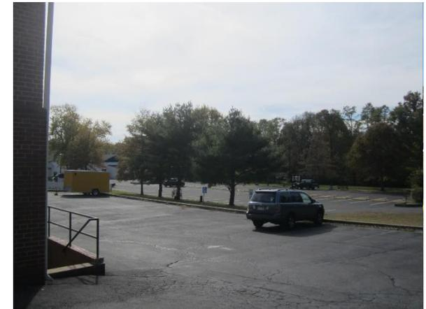
Parking spaces can be replaced with pervious pavement to capture and infiltrate stormwater. Bioretention systems can be installed to capture, treat, and infiltrate roof runoff. A preliminary soil assessment suggests that the soils have suitable drainage characteristics for green infrastructure.
