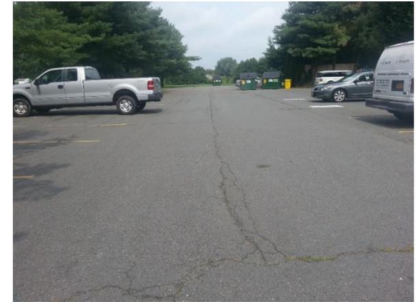
Bioretention systems can be installed to capture, treat, and infiltrate roof runoff. A row of parking spaces can be replaced with pervious pavement to capture and infiltrate stormwater. A preliminary soil assessment suggests that the soils have suitable drainage characteristics for green infrastructure.
