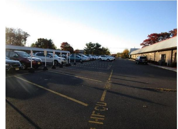
Rows of parking spaces can be replaced with pervious pavement to capture and infiltrate stormwater. A preliminary soil assessment suggests that the soils have suitable drainage characteristics for green infrastructure.
