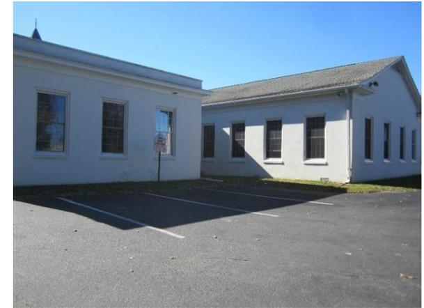
A bioretention system can be installed to capture, treat, and infiltrate roof runoff near the entrance to the church. Rows of parking spaces can be replaced with pervious pavement to capture and infiltrate stormwater. A preliminary soil assessment suggests that the soils have suitable drainage characteristics for green infrastructure.
